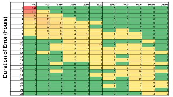
For e.g., there are 10 instances of 18-hour forecast error with a magnitude ranging from 4,000-6,000 MWh (hourly avg range of 222-333 MWh).
